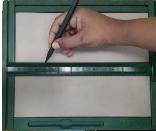
Figure 3.2b: Draftsman ruler aligned such that there is no gap between the ruler and sheet
