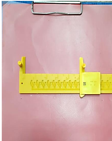
Figure 3.3: Immobilization System on the new metric system Squirrel ruler
