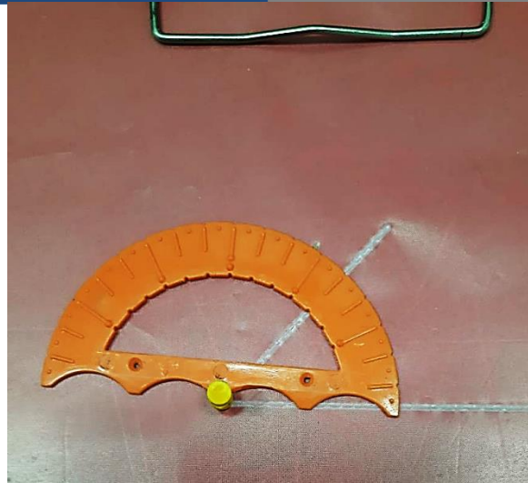
Figure 7.2: WT protractor aligned slightly off the baseline
