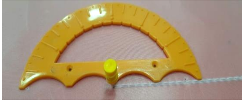
Figure 4.3b: WT protractor aligned correctly to the vertex pin and baseline
