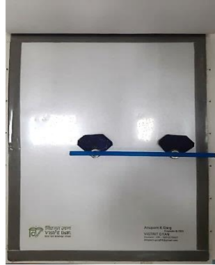
Figure 35: Two Point Markers with a Line Marker on them in the position to draw the baseline of an angle on the Garg board
