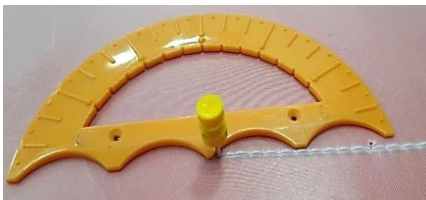
Figure 4.3a: WT protractor aligned incorrectly to the vertex pin
