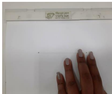
Figure 17: Puncturing holes at the end points with the Garg board
