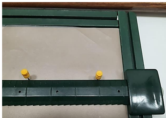
Figure 12: Smooth edge of Draftsman ruler touching plotted point pins
