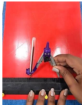
Figure 50: The Classmate compass being aligned for a specific measurement with the APH clip ruler on the Exam board
