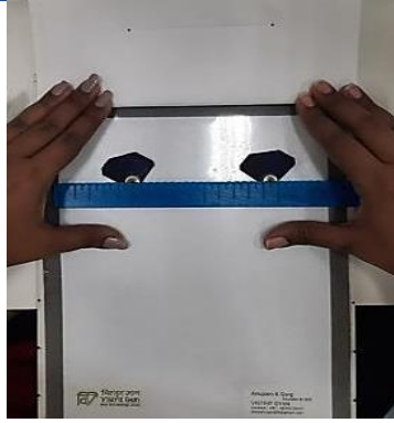
Figure 20: Paper pressed down onto the clip on the Garg board, thus making visible the point markers and ruler that were previously under the paper.
