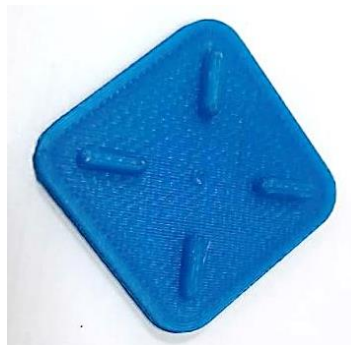
Figure 2.25: Line marker bridge
