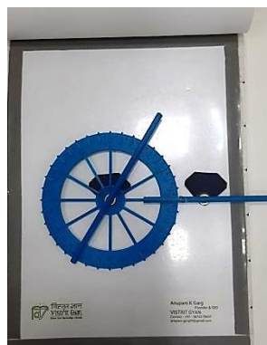
Figure 39: An extra line marker positioned from the 60-degree tactile marking on the Garg protractor towards the vertex
